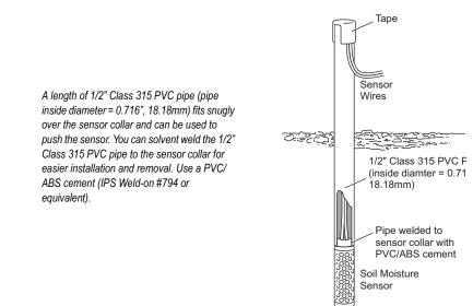
4. Carefully backfill the access hole with soil to eliminate any air pockets which could allow water to channel down to the sensor.
